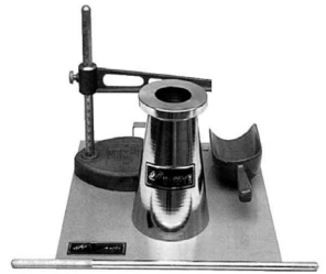
▲ Slump Test set
